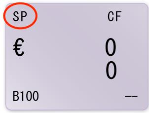
The machine sorts out the same denomination with first inserted note.
