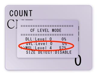
In COUNT Mode, machine can have simple detection function by adjusting MG Level. User can select 1~8 levels.
