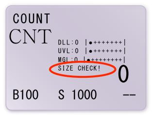
If SIZE DETECTION is enabled, machine can detect the different size note. When a note which has a different size (±5mm) from the first note is inserted, machine stops.
